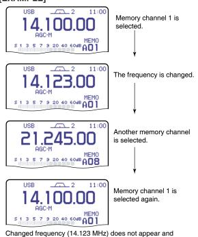
Changed frequency (14.123 MHz) does not appear and memorized frequency (14.100 MHz) appears instead.
